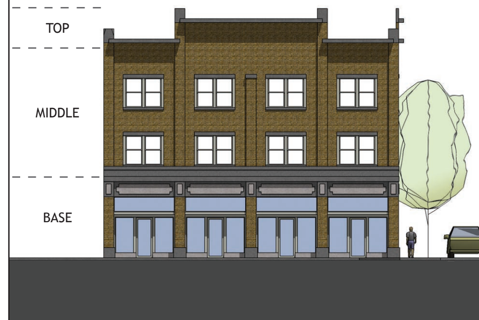
How the base, body and cornice system works on buildings of different heights. Above, a 2 story building; below, a 3 story building.
